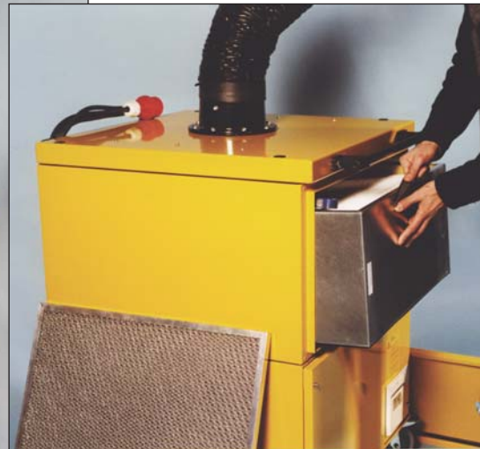
Front access makes the welding filter easy to remove.
