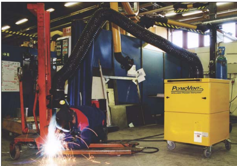
The PlymoVent Extraction arm can be rotated through 360° – reach everywhere!
